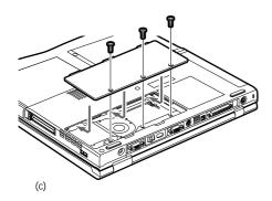
Figure 4-8 Removing a Memory Upgrade Module
